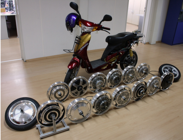
Figure 4 Scooter test unit with variety of motor types
