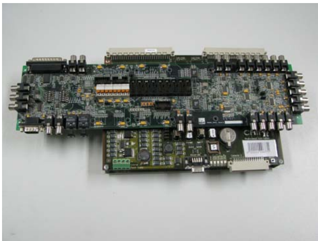
Photo of prototyping environment for multi channel audio IC
